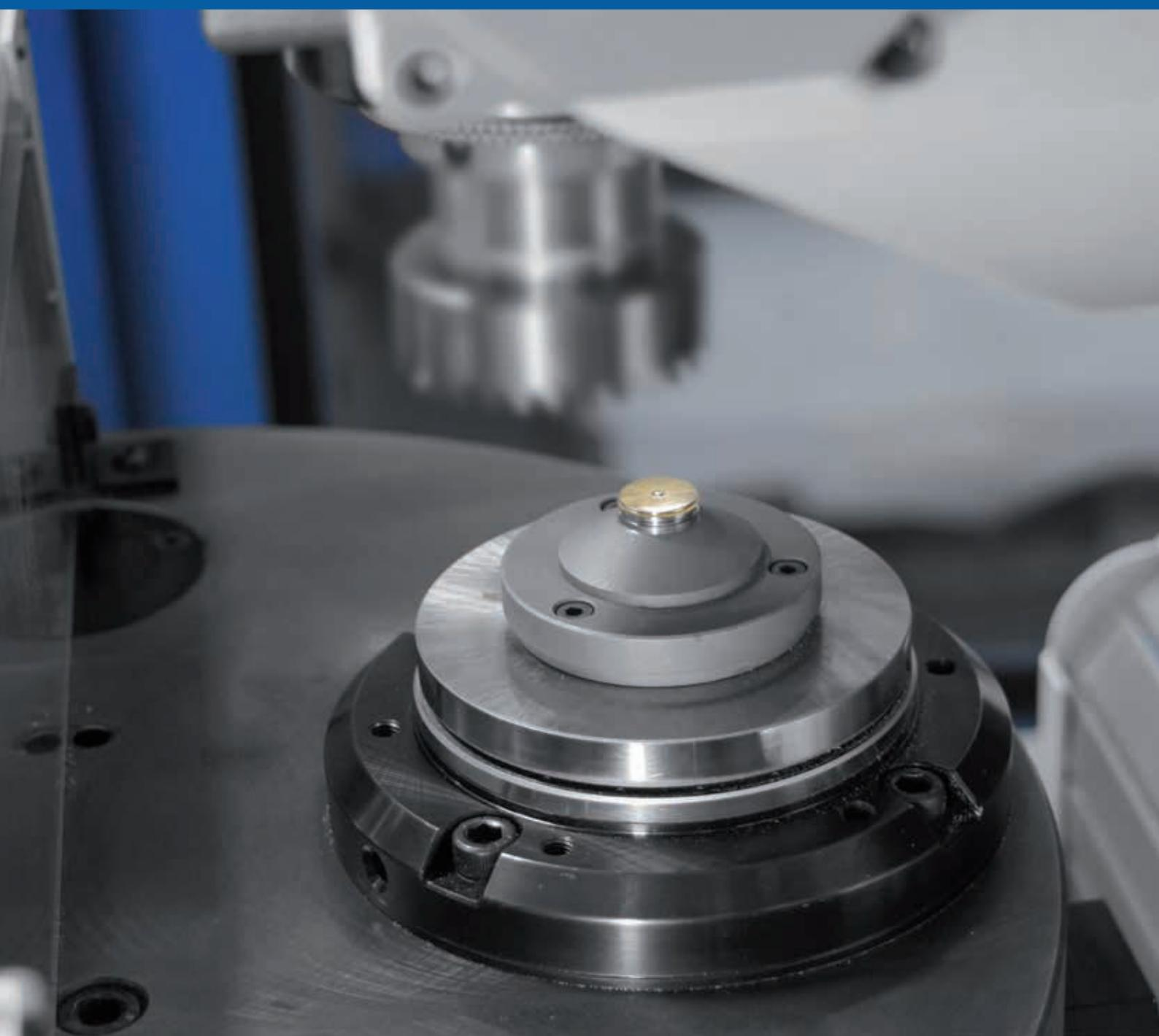
The SPEEDTOOL 100 is a high precision machining and micromachining with 4 axis. It's mainly dedicated to the machining of complex or high precision parts. This DECOR version is specialized in creation of watch decoration on all support.
