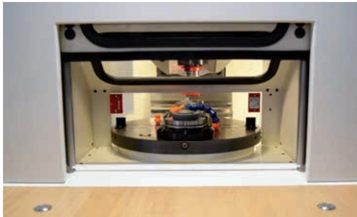
A rotary table allows loading in masked time. A double-walled door prevents the user to access the machining area during the cycle and thus allows a safety loading.
